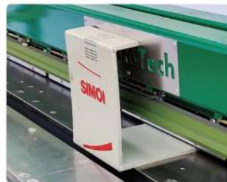
0 - 95° Bending by one sheet
