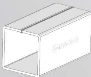
Bending (Non-Touch Welding)
