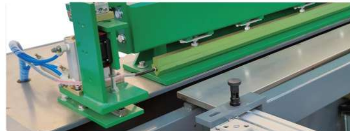
Optional: Heating Knife for Station 2/3/4
