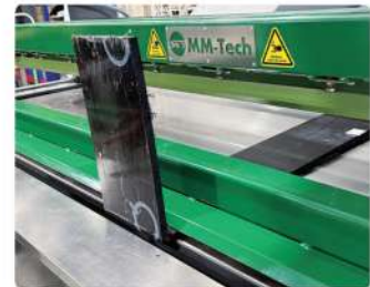
0 - 95° Bending by one sheet
