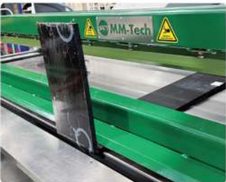
0 - 95° Bending by one sheet
