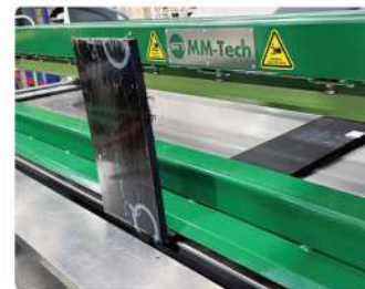
0 - 95° Bending by one sheet
