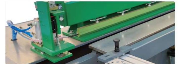
Optional: Heating Knife for Station 2/3/4
