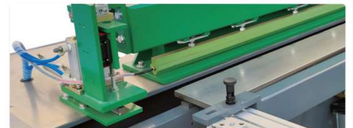
Optional: Heating Knife for Station 2/3/4
