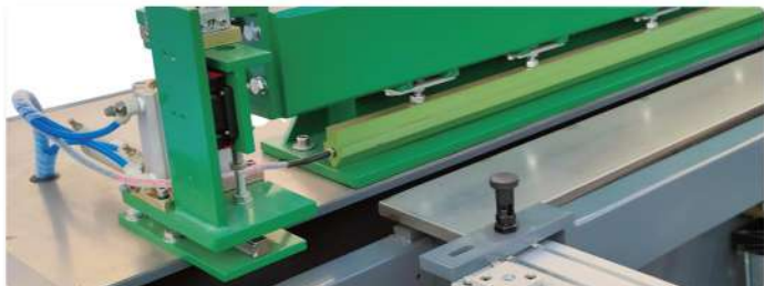
Optional: Heating Knife for Station 2/3/4
