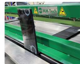
0 - 95° Bending by one sheet
