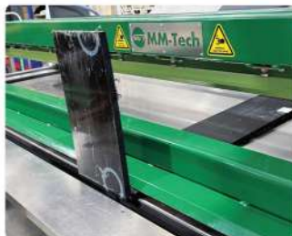
0 - 95° Bending by one sheet
