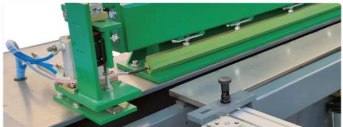
Optional: Heating Knife for Station 2/3/4
