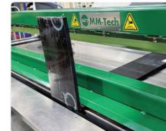
0 - 95° Bending by one sheet
