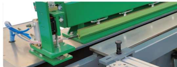
Optional: Heating Knife for Station 2/3/4
