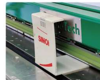
0 - 95° Bending by one sheet
