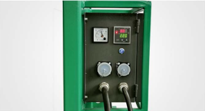
All connection sockets at the back of electrical cabinet
